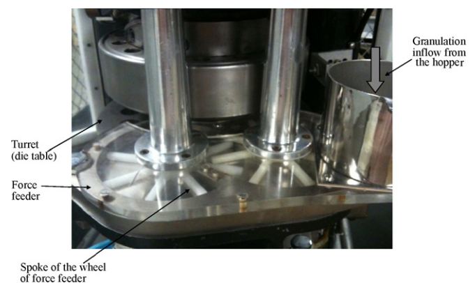
Fig. 8. Image of a force feeder (FF) used with the 16-station Betapress. The FF is shown in its position on the turret (TR). The FF shown is a closed chamber with two rotating wheels and an opening each for (a) the granulation inflow from the hopper through the receptacle shown on the right and (b) granulation outflow to the die cavities through openings on the bottom, that are aligned with the position of the dies on the turret. As the granulation passes through the FF, it gets filled into the die cavities in the turret, which rotates in a clockwise direction. The transparent top of the FF allows visualization of the spokes of the wheels of FF that rotate during its operation.
